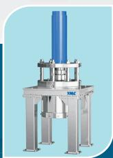
YMC provides dynamic axial compression columns suited for various separation scales such as laboratory-pilot- and industrial-scale. They are automated self-packing columns that allow for an easy, cost-effective refill of packing material that results in a column bed yielding superior durability and reproducibility. Dynamic axial compression (DAC) keeps the sorbent bed under constant compression throughout development of the column.
